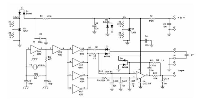
U3A is an oscillator using the ceramic resonator Y1. The output of U3C to U3F charges and discharges the capacitor to be measured at a 455kHz rate. The charge current flows through R8, and it is filtered and amplified by the differential amplifier U4. The discharge is made through D3. The average current in R8 is proportional to the capacitance.
